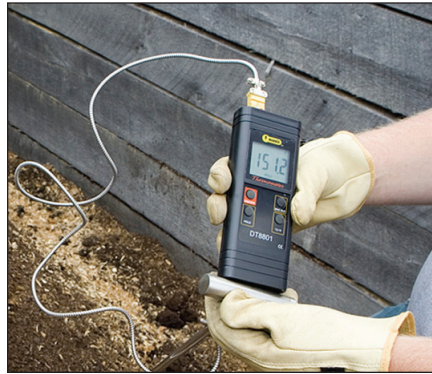
Figure 5. Example of an electronic thermometer. Note the temperature reading of 151°F.
