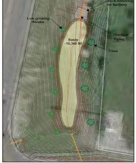
**Concept Plan:** *The concept plan illustrates approximate size of the proposed bioretention basin.*
