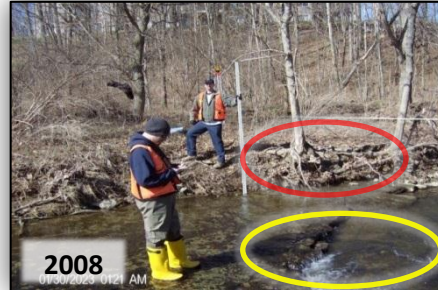
Also in the South Fork subwatershed (site SFG 5.3-DS), the erosive flow regime has caused the banks to enlarge, particularly the left bank, which has expanded more than 3 feet, resulting in the loss of two trees (red). It has also caused bedrock incision as the stream bed continues to deepen (yellow).
