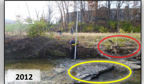
Also in the South Fork subwatershed (site SFG 5.3-DS), the erosive flow regime has caused the banks to enlarge, particularly the left bank, which has expanded more than 3 feet, resulting in the loss of two trees (red). It has also caused bedrock incision as the stream bed continues to deepen (yellow).
