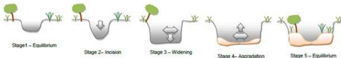
Figure 4-14: Channel Evolution Sequence in response to increased flows from urbanization, Adapted from Schumm et al. (1984) and Hawley et al. (2012).
