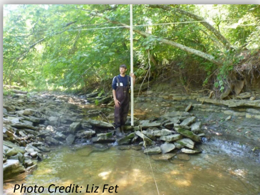
Figure 3-4: Hydrogeomorphic surveying at site ALF 0.1 - collecting cross section data
