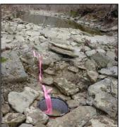
Sediment Mobility Monitoring: Data collection using cork gage, bed load sampler, and spray-painted particles confirms wetland performance.
