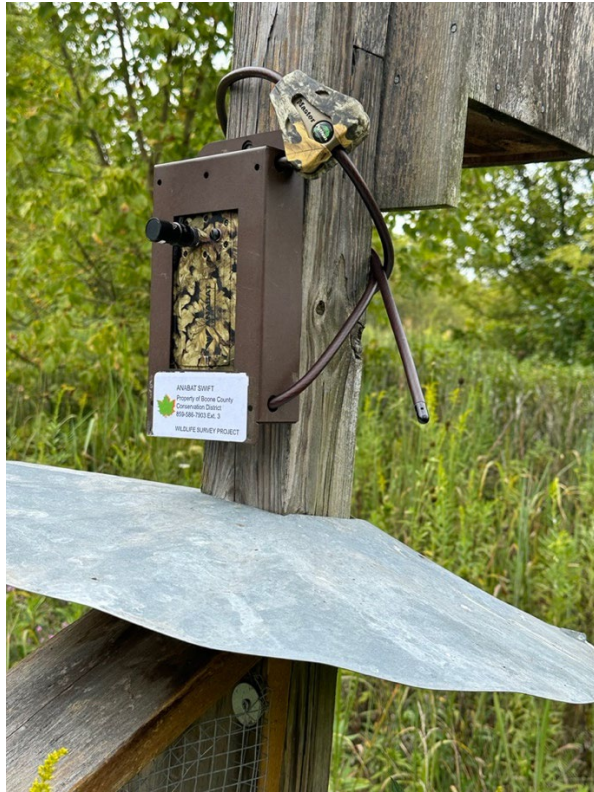
App. Figure 15. Anabat Swift Acoustic Monitoring Stationary Device by Titley Scientific, Omni-directional Ultrasonic Microphone US-O V3, Master Python Cable Lock (September 2023, Conservancy Park Bellevue)
